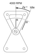
**TIP**: Rather than trying to move the sensor plate with the engine running, mark the location with a pen and adjust according to the mark with the engine stopped. Remember a 1 degree change to the sensor plate makes a 2 degree adjustment at the crankshaft. Use small adjustments and recheck with the strobe as above.
