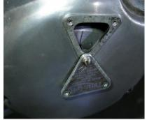
an early model engine or crankshaft. The crankshaft should now be at 38 degrees BTDC relative to the timing side cylinder on the compression stroke.
