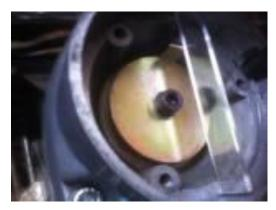
Using the plastic strip provided check for a 2 -3 mm air gap between the top of the rotor tab and the strip as shown here. **This gap is critical**. A smaller gap will result in damage to the rotor and sensors. As a guide, the thickness of the strip is 2mm. Increase the gap if required by filing the tab or adjusting the taper.
