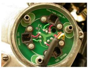
Feed the free end of the cable attached to the sensor plate through the hole in the bottom of the points cavity where the points wiring was originally located.
