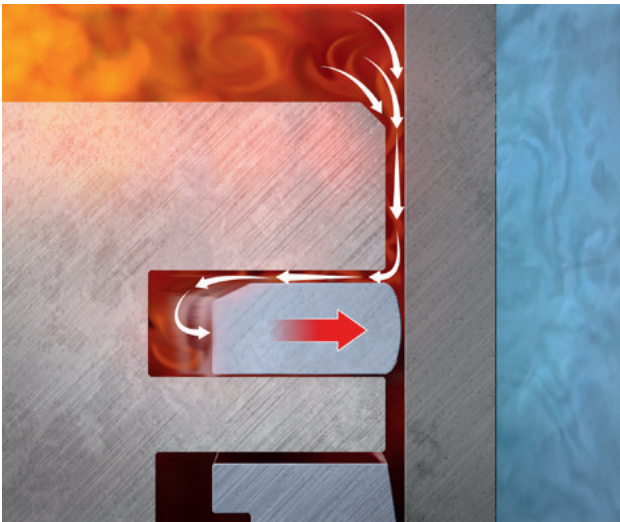
Fig. 1: Increase in contact pressure
