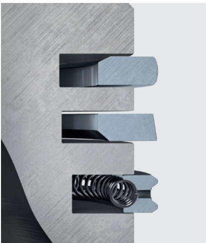
Fig. 2: Piston rings untensioned – twisting still ineffective
