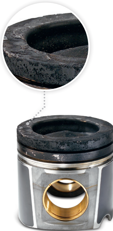
Fig. 3: Carbon layer on the top land
