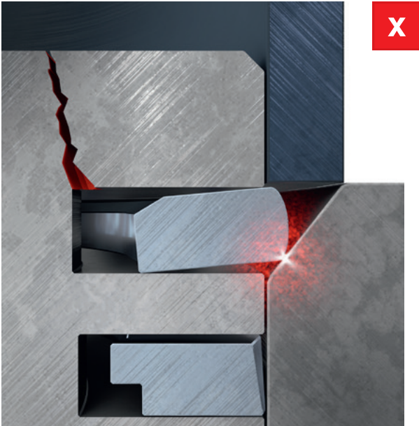
Fig. 1: Chamfer on the cylinder bore too large – the piston rebounds between the piston ring scuff band and cylinder during mounting and the piston becomes blocked
