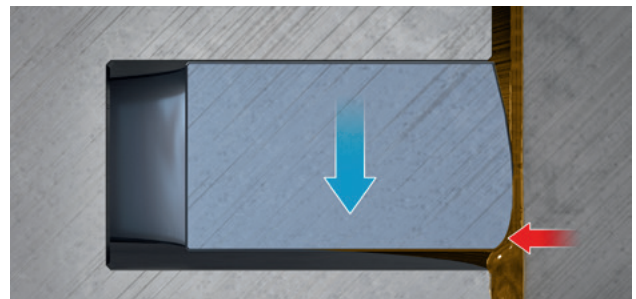
Fig. 5: Low floating in the downwards movement
