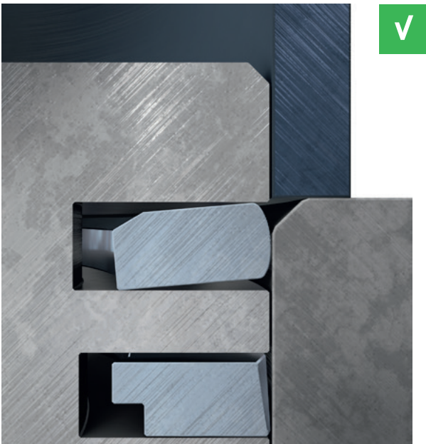
Fig. 2: Small chamfer on the cylinder bore – the piston ring slides over the gap
