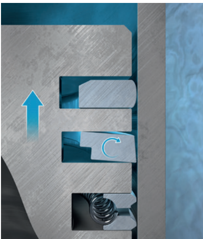
Fig. 5: Without combustion pressure
