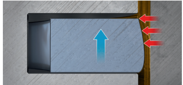
Fig. 4: High floating during the upwards movement
