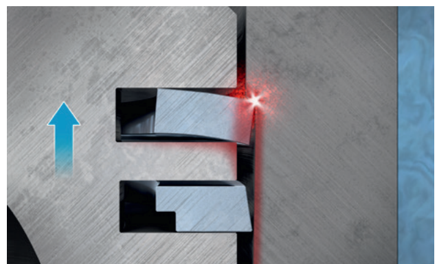
Fig. 3: Impact of the piston ring with the new piston
