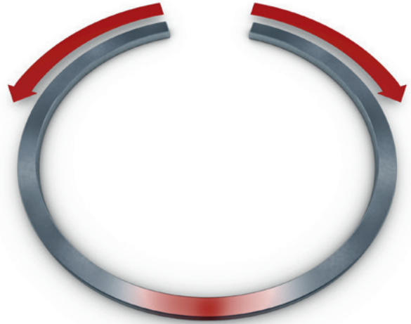
Fig. 1: Excessive spreading of the piston ring
