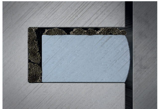
Fig. 1: Dirt deposit in the ring groove
