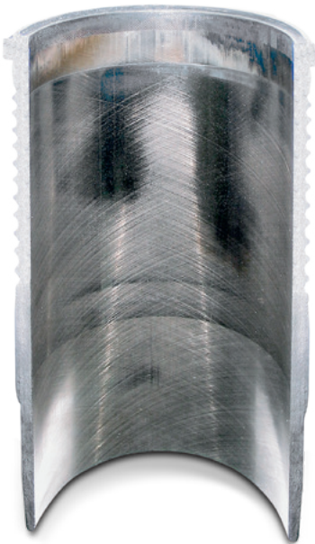
Fig. 2: Bright and polished areas in the top cylinder area
