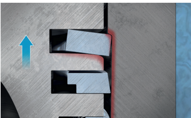
Fig. 2: Impact of the piston ring with the old piston
