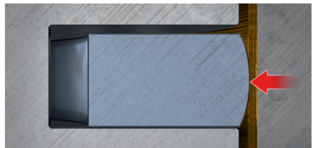
Fig. 2: Symmetrically crowned piston ring sliding surface
