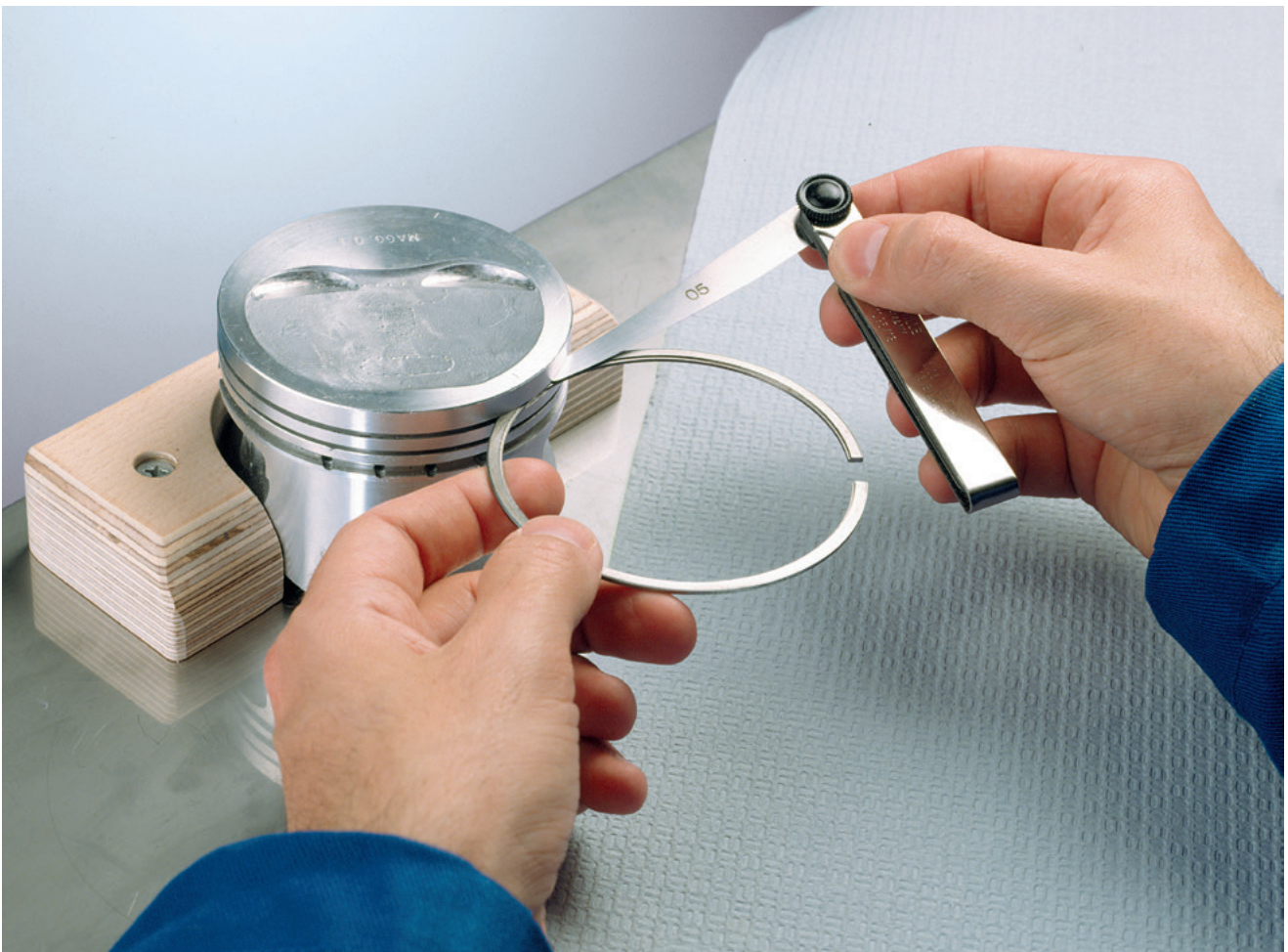
Fig. 1: Measuring the ring height clearance
