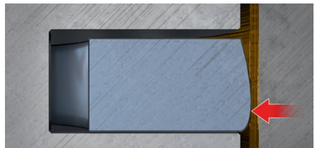
Fig. 3: Asymmetrically crowned piston ring sliding surface
