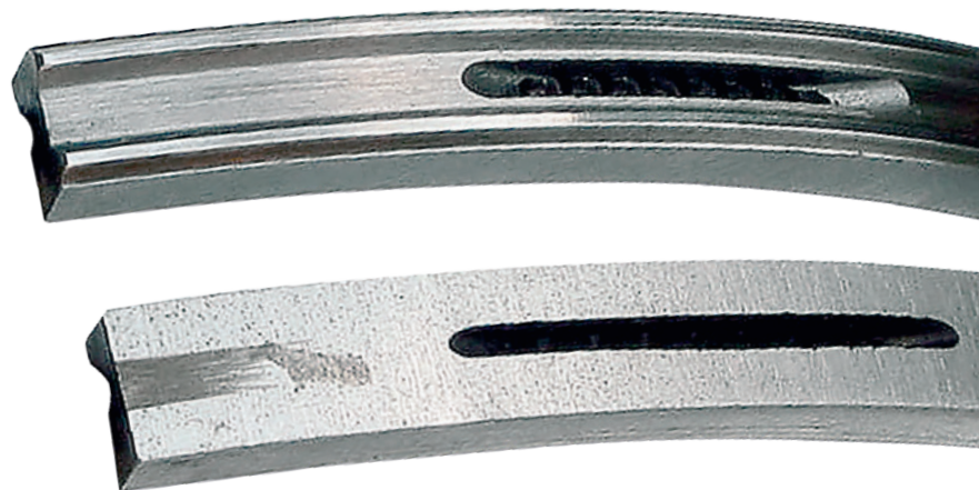
Fig. 3: New and worn oil control ring
