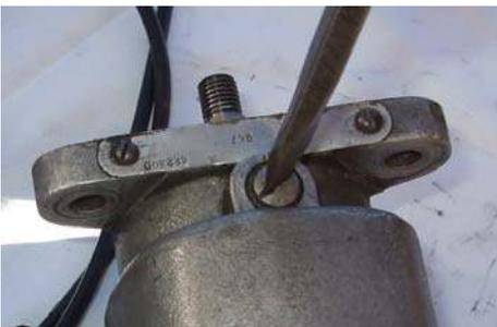
*On some magnetos, the earth brush is sometimes hidden beneath the name plate.*
