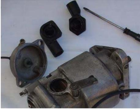
Remove the HT pickup(s) and contact breaker end cover.
