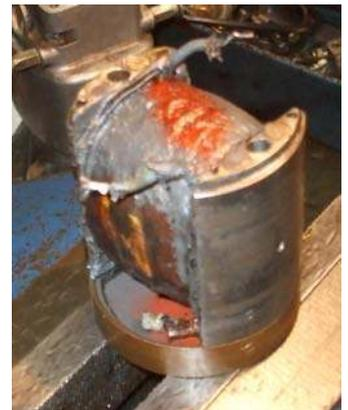
Having disconnected the wires, you can now separate the drive-end end-piece completely from the remainder of the armature.
