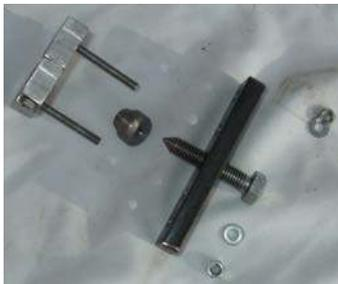
The pictures left and right show the components used for pulling the bearing inner race.
