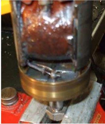
With the armature held in a vice as in the picture to the left, i.e. with the HT spike nearest you, you should see a wire in a sheath coming out of the left-hand side of the lower end of the bobbin. This is the common earth of the HT and LT windings.
