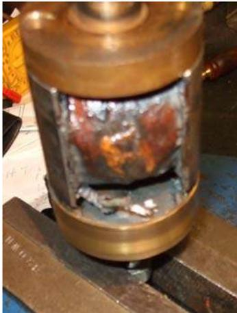
need to wiggle to wire with a pair of long-nosed pliers in order to free it. But be careful not to break the earth wire near its exit point from the bobbin. If you do break it there, the bobbin will need to be rewound.
