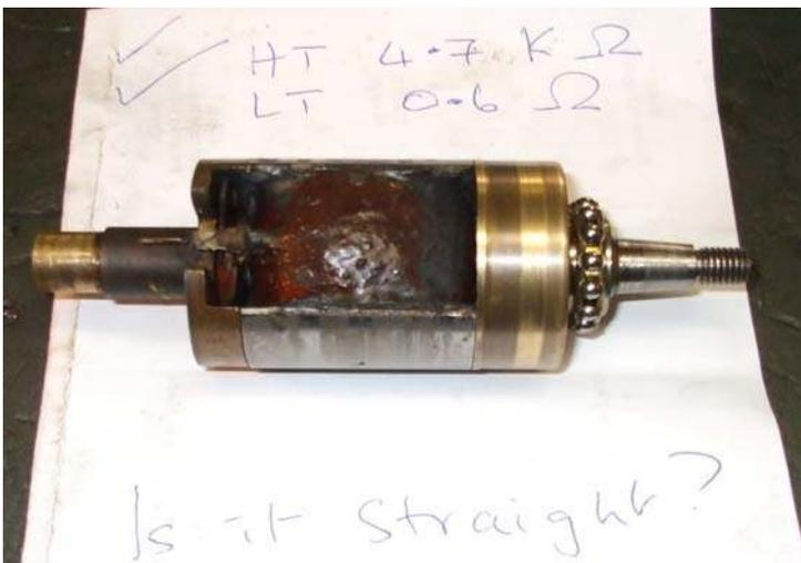
Now, using the scribe marks you made earlier, work out which of the two 5BA holes in the brass end-piece is going to have the earth wire connected to it, and block the other hole with a spare 5BA screw, silicone or other suitable material. This will prevent any grease from the drive-end bearing getting into the interior of the armature through the hole.
