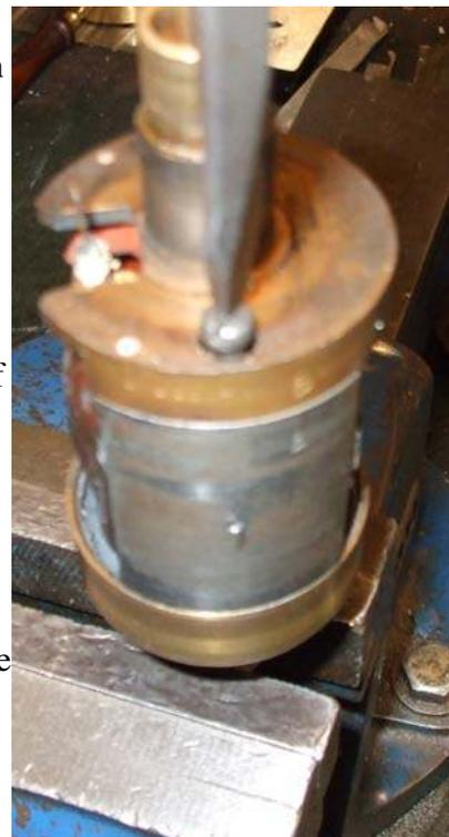
Then, the brass end-piece containing the condenser needs to be gently pulled from the bobbin. At this stage you do not need to separate them completely, just by about 5/16" (8mm).
