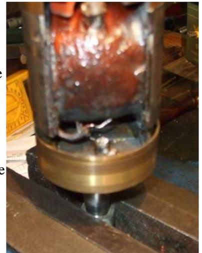
You may be able to see where it is connected to earth, for example by being soldered to the metal casing of an original Lucas condenser or its metal mounting bracket, or to a solder tag connected to the brass end-piece. If so, unsolder it. A decent soldering iron, say 50W, is needed to get the joints to part. Try to concentrate the heat on the joint. Steady hands are needed, as the coil and the wires leading from it won't respond well to excess heat. Once the solder is molten, you may
