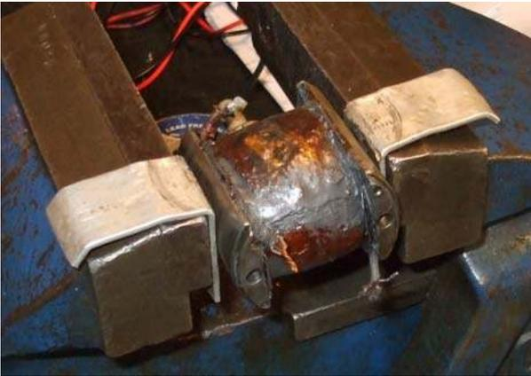
You may, however, need to (a) trim back some of the original sheath, (b) bare the wires of their insulating coating or old solder, (c) twist them together, (d) trim them and (e) solder them together, prior to sheathing them in two layers of adhesive-lined heat-shrink sleeving.
