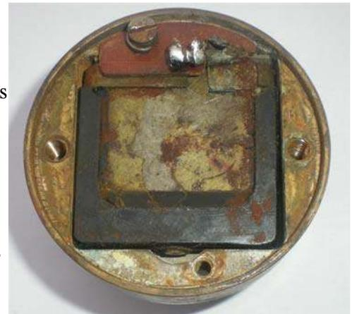
Fit the old condenser back into the end-piece, the same way round as before, and
