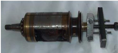
Possibly one or more shim washers can then be removed (note and keep safe), as too can the oil flinger which prevents any oil getting onto the slip ring.
