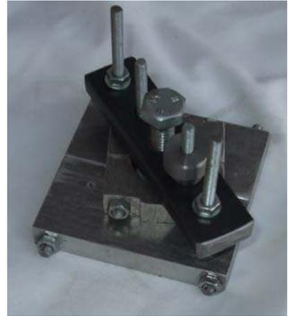
It is sometimes possible to remove the slip ring by hand without damaging it, but it is far safer to use a special puller as is also included in the Toolpack.
