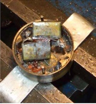
Clean up the end-piece. You should have found one, and possibly two, short 5BA screws in there, screwed into the smaller holes adjacent the 2BA holes for the long through-screws. Retain it/them.
