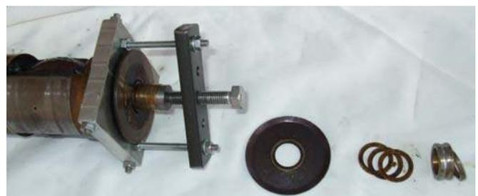
With the slip ring pulled, note the spike of the HT coil, which fits into a very snug hole in the boss on the rear of the slip ring. **Take extreme care not to bend the HT spike unintentionally.**
